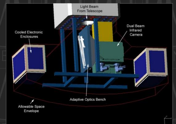
The future of extra-solar planet detection at Gemini observatory! NICI employs a dedicated AO system along with a dual channel IR imager and a variety of pupil masks, dichroics, filters, neutral splits, and polarizing elements. This will be the only instrument in Gemini's suite dedicated to extra-solar planet detection.
