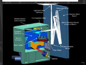
This diagram shows the AO bench, dual channel IR imager, and the internal optics that comprise NICI.
